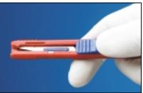
To permanently retract the blade move the slider past the 'safe' position into the permanent notch at the end of the scalpel.
